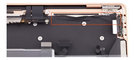
1. Inspect both sides of the top case for damage to the tape. If the tape looks like these examples, skip to step 7.
