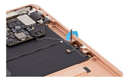
11. Align the screw holes on the battery tray over the alignment pins and lower the battery onto the top case.
