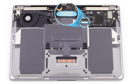
27. Turn over the computer. Use the flat end of the black stick to lift off the gap offsets and Kapton tape.
