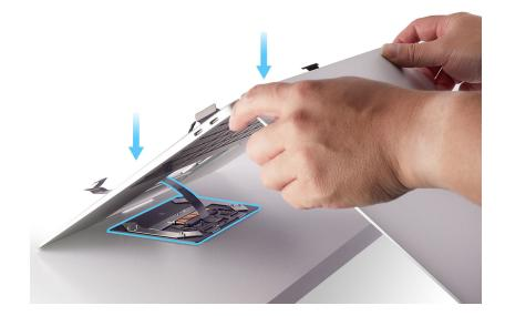
6. Slide the end of the IPD flex cable into the connector. Then flip down the locking lever.
