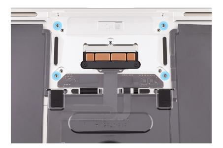
10. Turn over the computer. Insert one gap offset in each of the four corners of the trackpad. Then secure each gap offset with a piece of Kapton tape.
