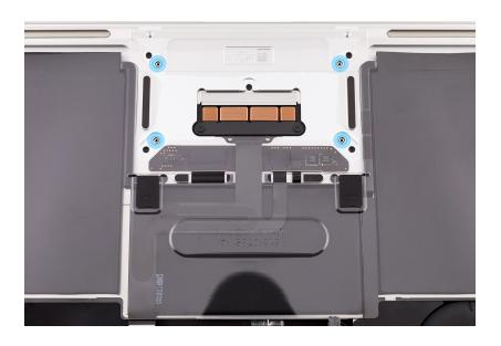
22. Hold the battery cover by the edges and lift it off the top case.
