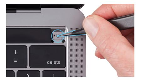
5. Set two Y-shaped alignment tools in the Touch ID board opening in the top case as shown. Secure the Y-shaped tools in the corner edges with Kapton tape.
