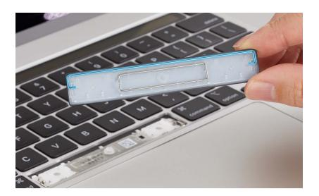
Position the keycap in the well and insert the top link bar into the metal hooks that are on each side of the well.
