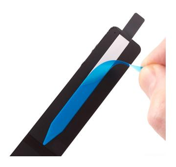
1. If you're reinstalling the existing speakers, peel the adhesive backing off the speaker adhesive strips.
