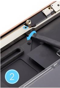
4. Repeat this motion below the other three screw holes to release the antenna module from the tape.
