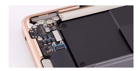
4. Place the flat end of the black stick under the left speaker flex cable to loosen the adhesive and peel the flex cable from the logic board. Then use the black stick to lift the end of the flex cable off the connector.
