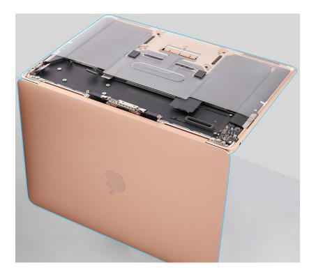
2. Use the T8 screwdriver to remove the six T8 screws (923-03997) from the display hinges.
