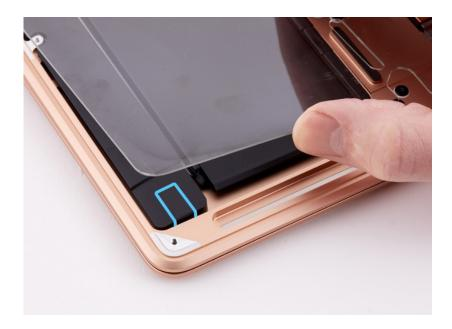
6. Use the T3 screwdriver to reinstall the T3 screw (923-03850). Then lower the corner of the battery cover.
