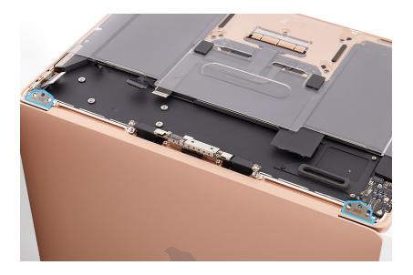
2. Ensure that the TCON board is inside the top case.
