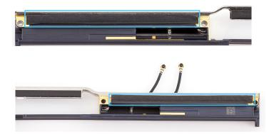
8. If one or both of the gaskets are wrinkled (1), use the flat end of the black stick to smooth them (2). Then skip to step 13. If one or both of the gaskets are torn (3), use ESD-safe tweezers to remove the gaskets.
