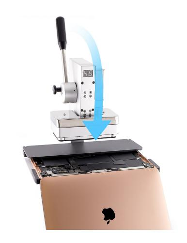
19. Wait until the timer on the iPhone display press beeps (1). Pull down the lever slightly and pull out the release knob (2). Then lift the lever (3).
