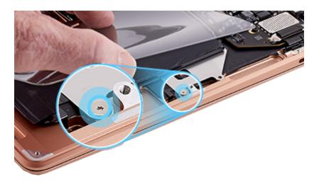
11. Repeat step 10 to remove the T3 screw from the battery tray on the other side. Then continue to step 12.
