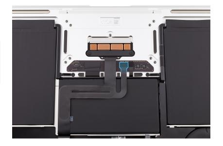
7. Place the battery cover on the battery and press the black tabs into the clips on the top case until you feel a click.
